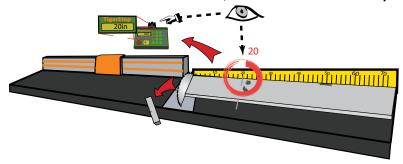
The operator feeds stock to the TigerStop®. When he reaches the first defect he cuts it out and enters the next usable clear length. He continues to make cuts until stock completion, only moving material and cycling the saw.
