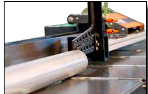
Pneumatic Tube Gripper
